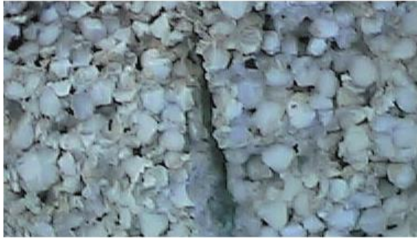
Perfect breakage, most beads adhered
